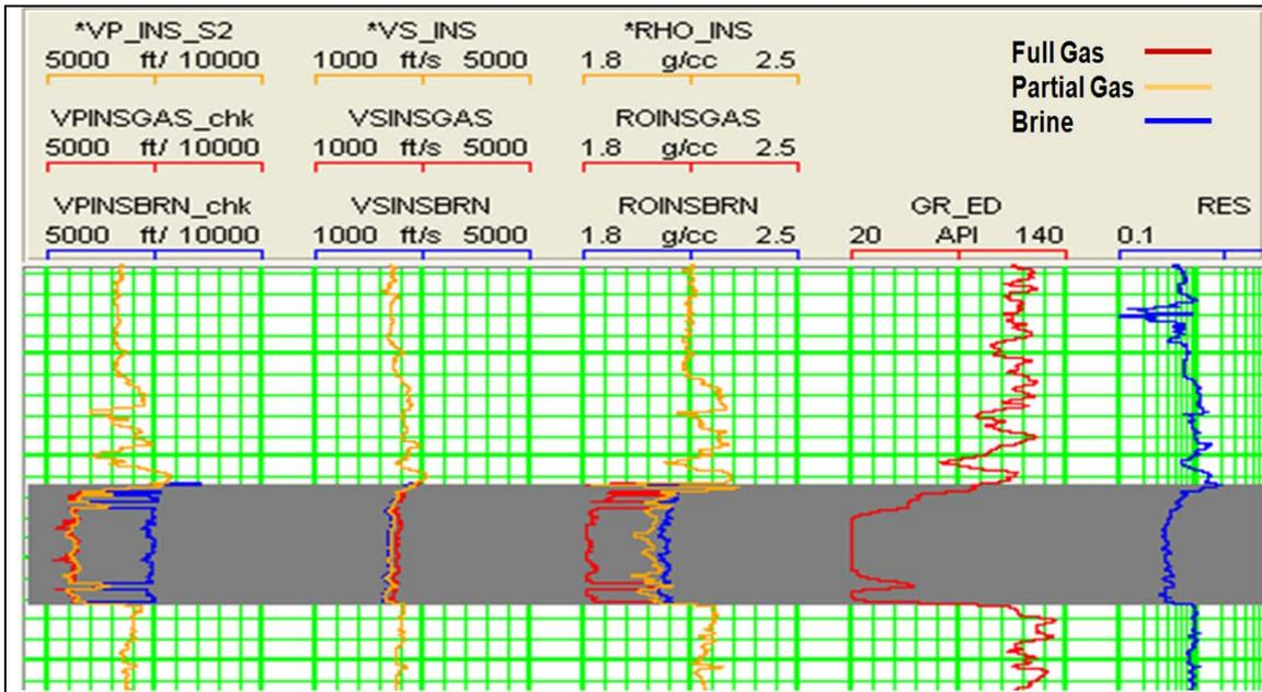
Figure 1: Fluid replacement results. The effect of the fluid type and saturation changes the well log response. Track 1 shows Vp or P-wave velocity, track 2 is Rhob or density and track 3 is Vs or S-wave velocity. In the first 3 tracks: Red, orange and blue colors represent log response for full gas, partial gas sand and wet sand. The GR is displayed in track 4 and the in situ resistivity in track 5. Notice that the in situ case is equivalent to the partial gas saturation case.
