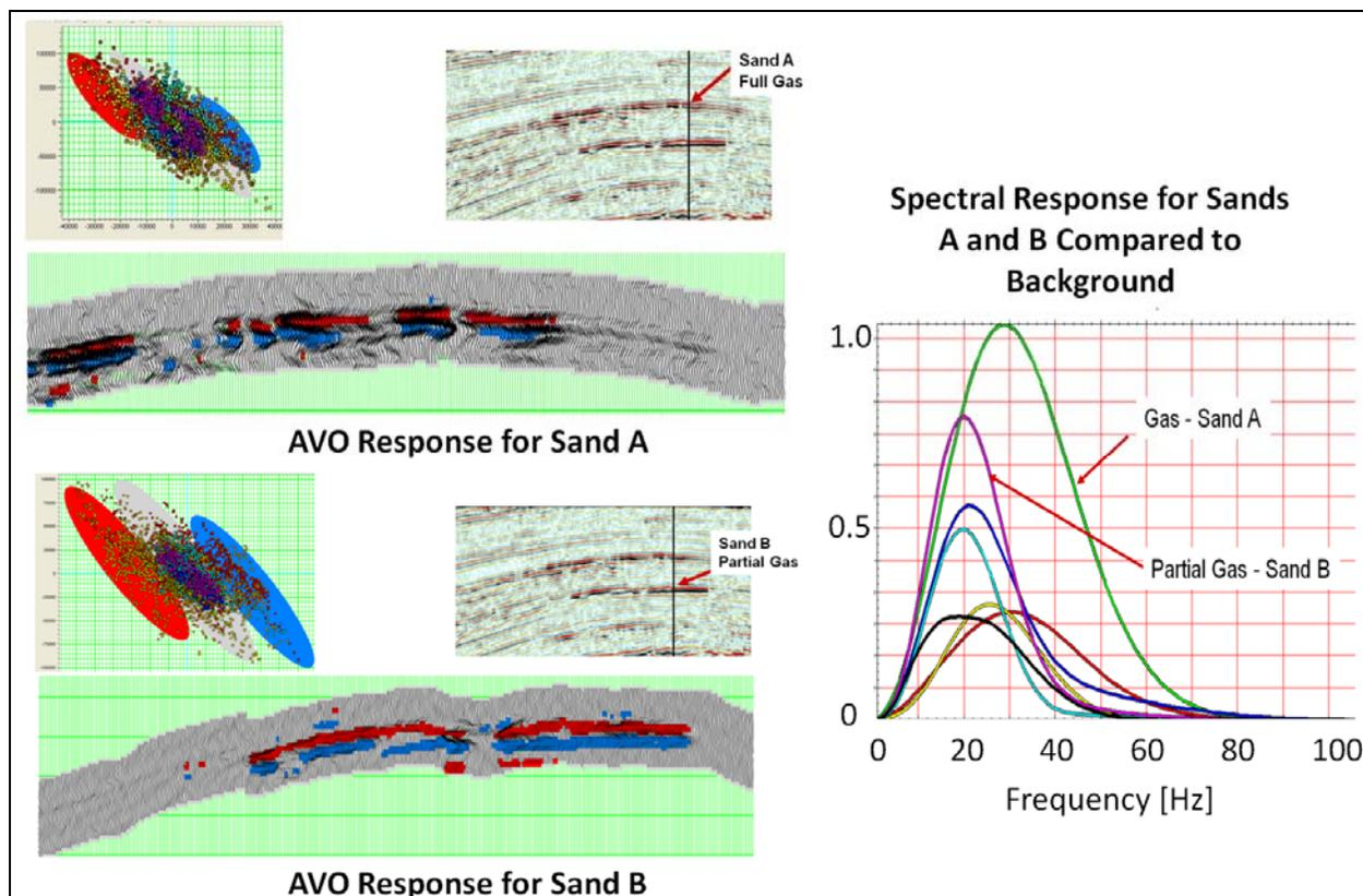
**Figure 4: AVO and Spectral Analysis in Calibration Area.** AVO crosplothing technique identifies clearly the presence of gas in the area. The spectral response for the fully saturated gas sand (sand A) shows a spectral response different to the response of the partially gas sand (sand B). The spectral response in the full gas case is wider in bandwidth while the spectrum (bandwidth) of the partially saturated gas sand (Sand B) is more comparable to the background.
