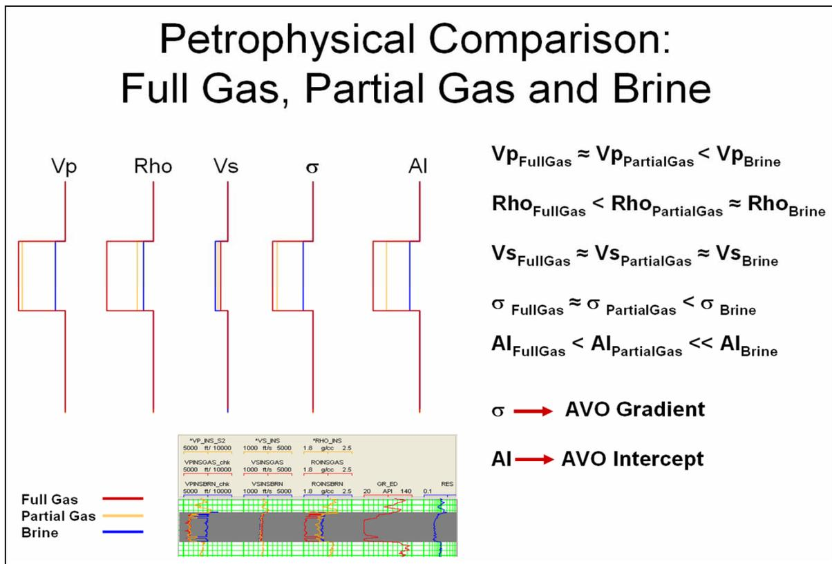
Figure 2: Sketch showing petrophysical properties for sand filled with different fluid types. Vp = P-wave velocity, Rhob is density, Vs is S-wave velocity, next track is Poisson's ratio and AI is impedance. Red, orange and blue colors represent log response for full gas, partial gas sand and wet sand. The bottom part is an insertion of figure 1 that shows the data used to generate the sketch.
